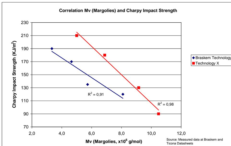
Figure 6 – Correlation between Mv (Margolies) and Charpy Impact Strength using Braskem production technology (blue) and a different technology (red).
