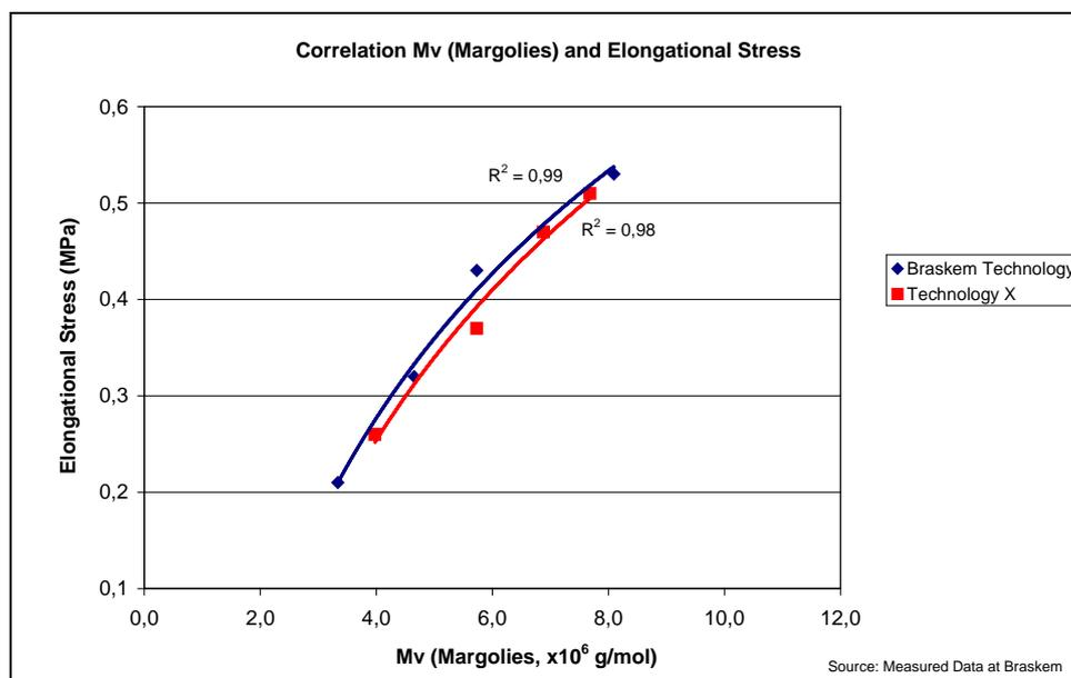
Figure 3 – Correlation between Mv (Margolies) and Elongational Stress using Braskem production technology (blue) and a different technology (red).
