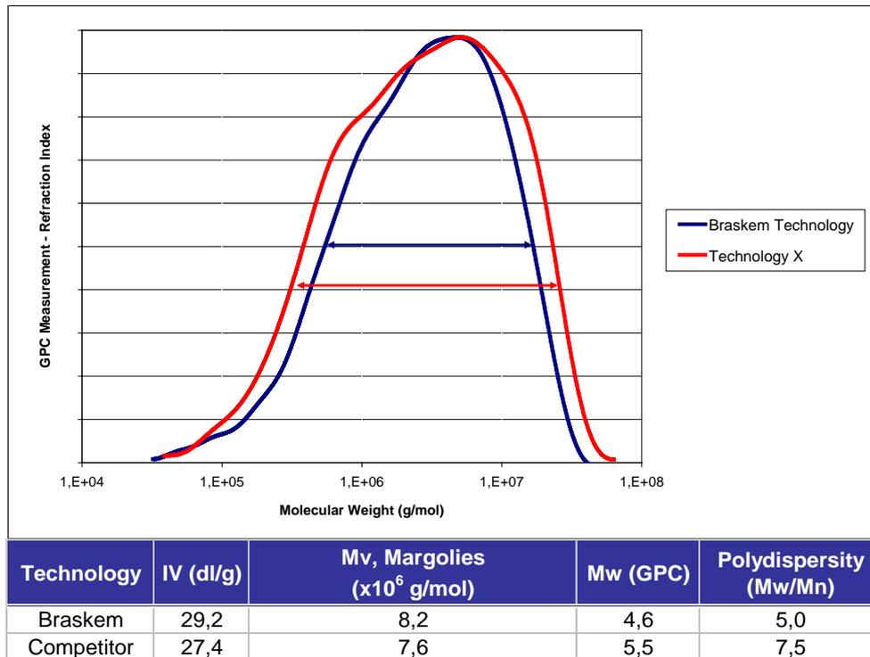
Figure 5 – Molecular weight distribution obtained from GPC for UHMWPE samples produced using Braskem production technology (blue) and a different technology (red).
