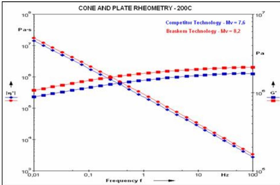
Figure 7 – Shear viscosity ( $\eta$ , [Pa.s]) and storage modulus ( $G'$ , [Pa]) obtained from cone and plate rheometry for UHMWPE samples produced using Braskem production technology (red) and a different technology (blue).
