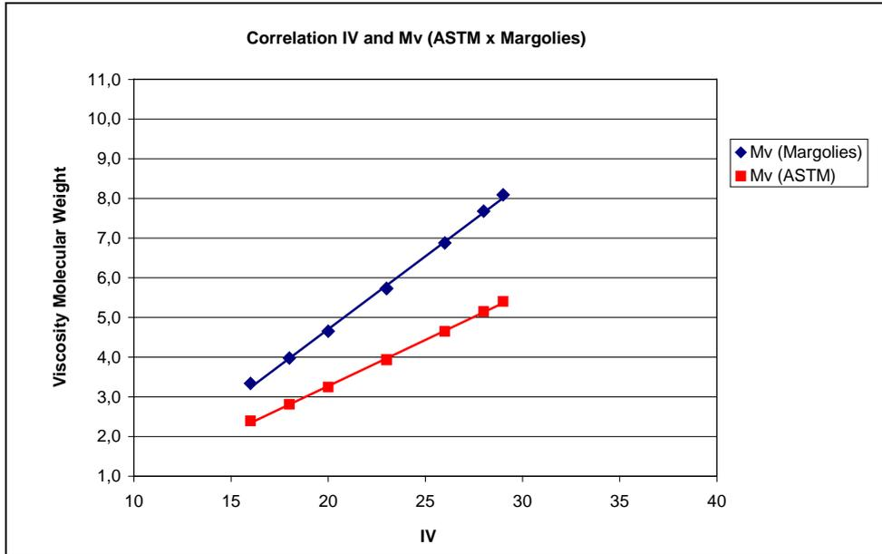
Figure 1 – Correlation between IV and Molecular Weight using Margolies’ Equation (blue) and ASTM Equation (red).
