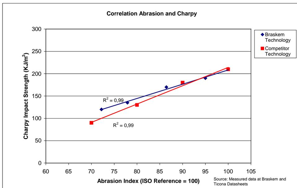
Figure 9 – Correlation between Abrasion Index and Charpy Impact Strength using Braskem production technology (blue) and a different technology (red).
