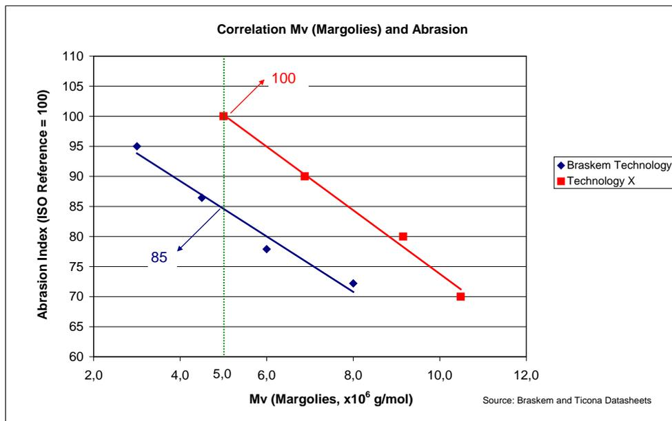
Figure 4 – Correlation between Mv (Margolies) and Abrasion Index using Braskem production technology (blue) and a different technology (red).
