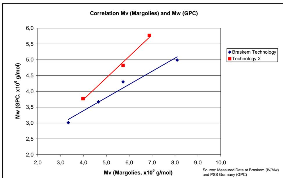
Figure 2 – Correlation between Mv (Margolies) and Mw (GPC) using Braskem production technology (blue) and a different technology (red).
