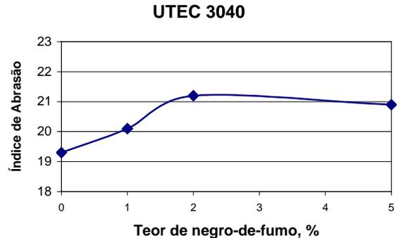
**Figure 12:** Influence of the CB concentration in the abrasion index of UTEC
