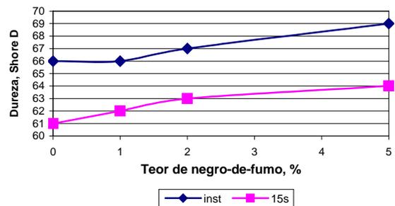
**Figure 4:** Influence of the CB concentration in the Shore Hardness of UTEC 3040
