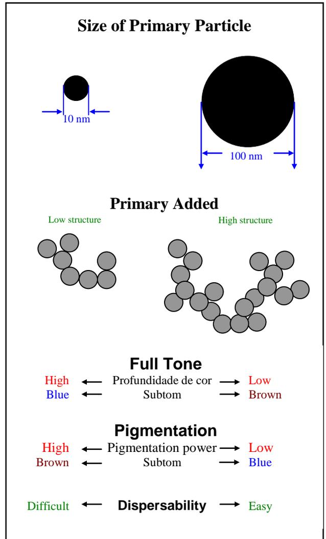
**Figura 1:** The effects of the size of primary particles and the structure of the carbon black pigments in the color depth, pigmentation power e subtom in plastics.
