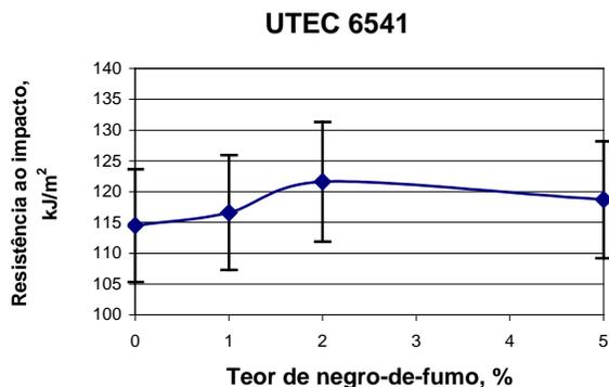
**Figure 11:** Influence of the CB concentration in the resistance of the impact of
