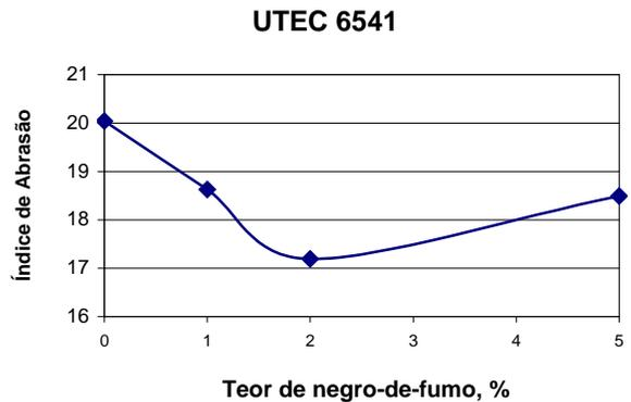
**Figure 13:** Influence of the CB concentration in the abrasion index of UTEC 6541
