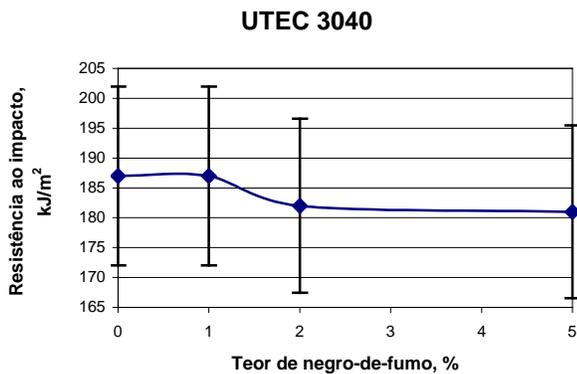
**Figure 10:** Influence of the CB concentration in the resistance of the impact of
